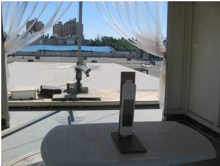
Figure 7. Radiated Emission Test, 200-1000MHz
