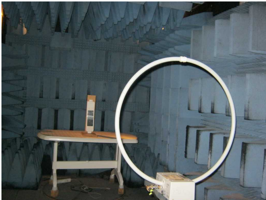
Figure 5. Radiated Emission Test, 0.009-30MHz
