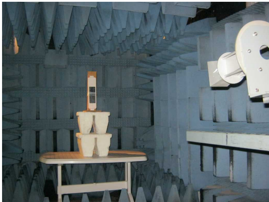
Figure 9. Radiated Emission Test, 18-26.5GHz
